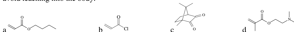
Figure 3: Structures of the adhesive a) comonomer, BA, and b) functionalization group, AC, and the photoinitiating system c) initiator, CQ, and d) co-catalyst, DMAEM.
